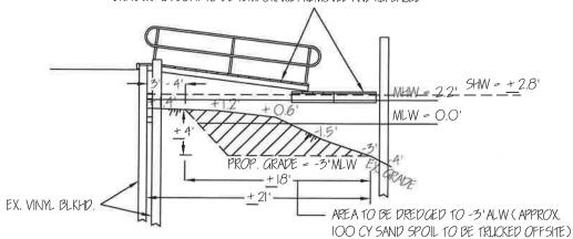
NOTE: OVERALL PROPOSED DREDGE SLOPE = 2:9 (MIN. 1:1)
